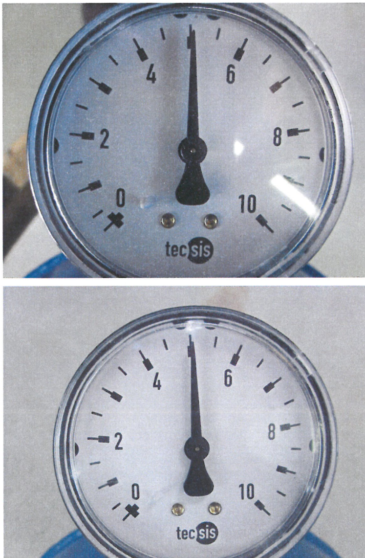
Figure 4: Tightness test with compressed air (5 bar) filled pressure bell at 23 °C (above: manometer display at the beginning of the test at 04/18/2011 07:45; below: manometer display at the end of the test at 04/19/2011 10:10)
