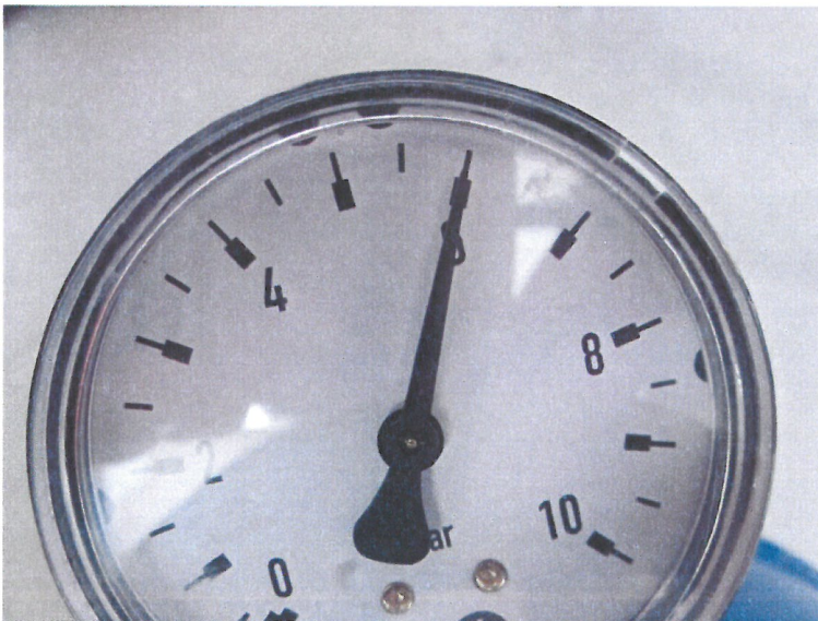
Figure 5: Tightness test with compressed air (6 bar) filled pressure bell at 23 °C (above: manometer display at the beginning of the test at 04/19/2011 11:30; below: manometer display at the end of the test at 04/20/2011 11:30)
