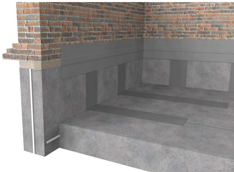
An underpinned structure with waterproofing to the concrete joints.
